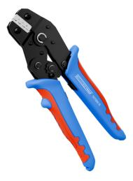
MULTI-CRIMP was developed for the process-safe crimping of various electrical connectors. The crimping tool has a ratchet mechanism with a blocking device to ensure a consistently high crimping quality and results that can be precisely repeated. The mechanism only opens the tool when the crimping process is complete. An emergency release has also been integrated into the handle, which opens the crimping tool in the event of misuse.
