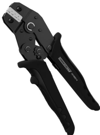
MC4-Crimp has been specially developed for the process-safe crimping of MC4 connectors on PV systems. The crimping tool has a ratchet mechanism with a blocking device to ensure a consistently high crimping quality and results that can be precisely repeated. The mechanism only opens the tool when the crimping process is complete. An emergency release has also been integrated into the handle, which opens the crimping tool in the event of misuse.
