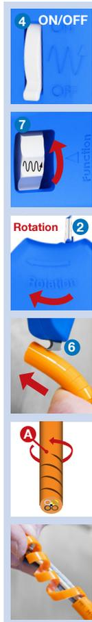
1. Adjust the cutting depth for the respective cable
