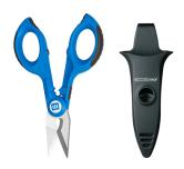
The scissors can be used for cutting and stripping Cu/Al wires and crimping wire end ferrules from 0.5 - 4 mm². The stainless blades made of high-quality INOX steel are hardened to 55 HRC and therefore very wear-resistant. The fine micro serration of the blades enables flush and slipfree cutting, resulting in a very precise cut. The non-slip 2-component handles made of impact-resistant fibreglass-reinforced plastic ensure safe working.
