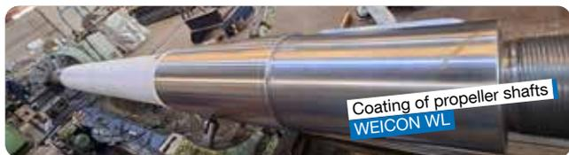
Coating of propeller shafts
