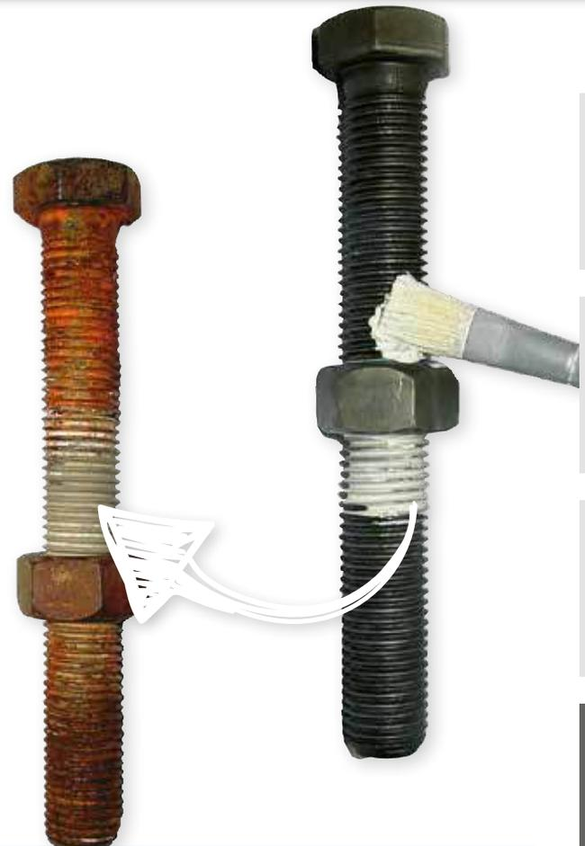
Due to the special formulation and the very fine grinding of the solids contained in WEICON Anti-Seize, irregularities in the protected surface are completely filled – even to a layer thickness of only 12 µm. Only a perfectly sealed surface guarantees a reliable protection against corrosion. An additional sealing effect thus results for special applications, such as flange connections.
