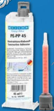
Due to its slightly higher viscosity, WEICON Easy-Mix PE-PP 45 compensates bonding gaps of up to 1 mm and, thanks to the fillers (glass beads) contained in the adhesive, guarantees adhesive joint of at least 0.20 mm.
