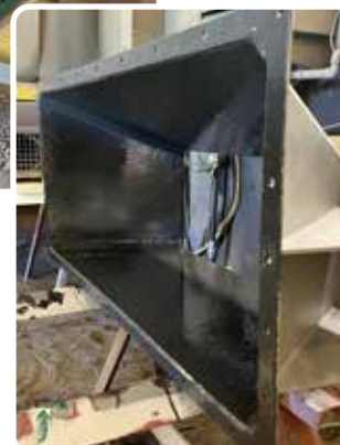
Triple coating of chutes WEICON GL-S WEICON Ceramic HC 220
