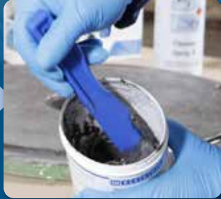
Mix resin and hardener thoroughly and bubble-free
