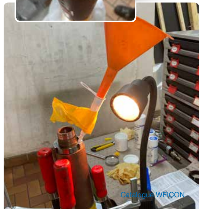
Interstitial grouting on a pipe-in-pipe system for electrical insulation WEICON Casting Resin MS 1000
