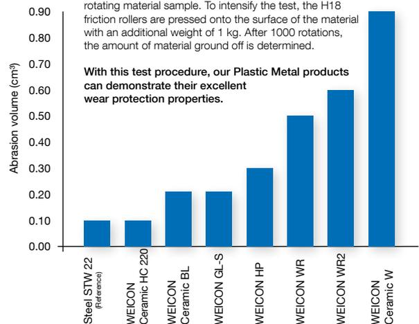
With this test procedure, our Plastic Metal products can demonstrate their excellent wear protection properties.
