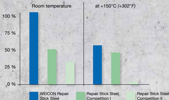
Adhesive strength of Repair Stick Steel
