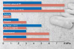
Specification of the test specimen: Standard: DIN EN 1465 Curing: Adhesive surface: 12.5 mm x 25 mm Adhesive thickness: 0.2 mm
