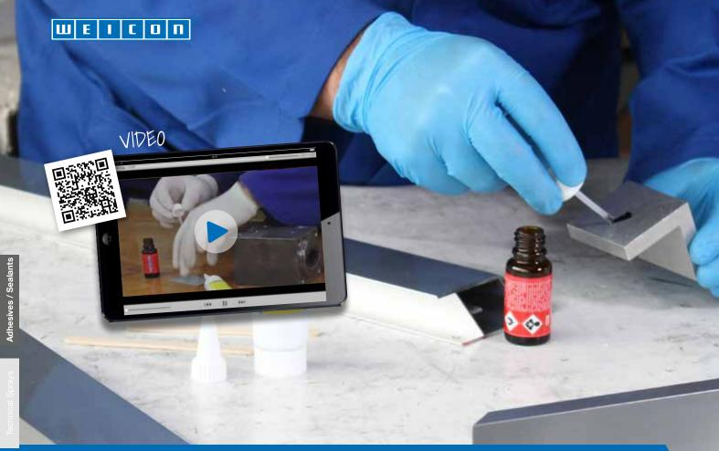
WEICON RK-1300/1500 are 2-component systems based on methacrylate, which cure fast at room temperature. Both systems are processed in the "no-mix" procedure, i.e. a mix of both components (adhesive and activator) is not necessary.
