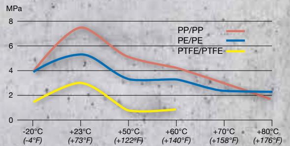
Strength development of WEICON Easy-Mix PE-PP 45 on tensile shear test samples compliant with DIN EN 1465
