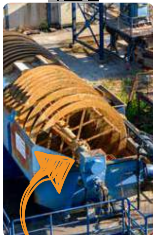
Lining and repair of chutes WEICON Casting Resin MS 1000 WEICON WR2 WEICON HP
