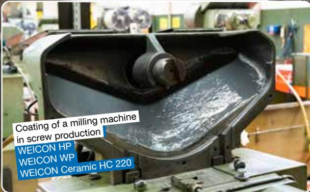
Coating of a milling machine
