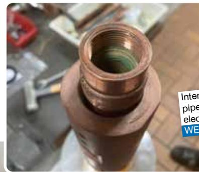
Interstitial grouting on a pipe-in-pipe system for electrical insulation | WEICON Casting Resin MS 1000
