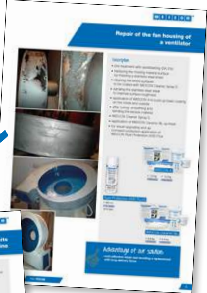
Repair of the fan housing of a ventilator
