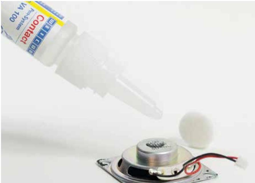
contamination such as oil, grease, dust and dirt can be removed with detergents such as special surface cleaners. The following applies: the cleaner the surface, the better the results you are aiming for.
