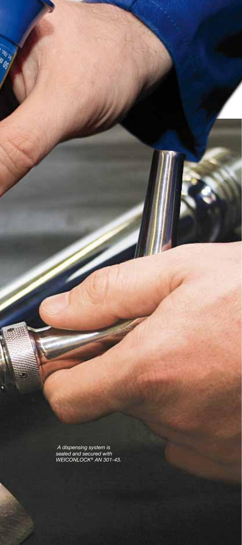
*A dispensing system is sealed and secured with WEICONLOCK® AN 301-43.*
