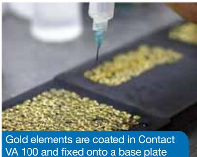
Gold elements are coated in Contact VA 100 and fixed onto a base plate
