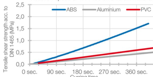
Reaction speed of VA 1408 on different materials
