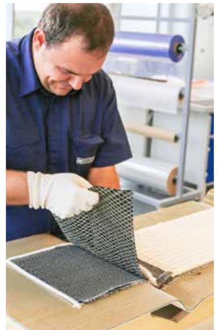
First, Mike cut the sandwich core, the fibres as well as all other support materials to the right shape. In order to do so, extra sharp scissors were needed, like our WEICON Cable Scissors No. 35, as the carbon fibres are very rigid.
