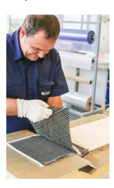
First, Mike cut the sandwich core, the fibres as well as all other support materials to the right shape. In order to do so, extra sharp scissors were needed, like our WEICON Cable Scissors No. 35, as the carbon fibres are very rigid.
