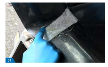
**Step 4:** Then apply another layer of the adhesive generously on top of the glass fibre tape. It's best to remove spare, non-cured adhesive immediately with our WEICON Surface Cleaner.
