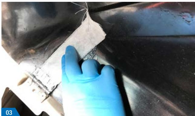
**Step 3:** Place the glass fibre tape right on top of the adhesive and make sure to cover the whole crack.
