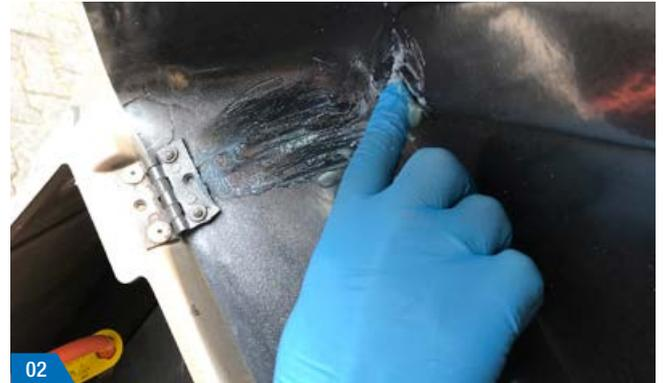
**Step 2:** Apply the adhesive evenly to the inside of the gas locker box over and around the crack.
