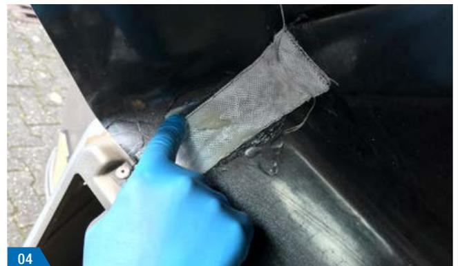
**Step 4:** Then apply another layer of the adhesive generously on top of the glass fibre tape. It's best to remove spare, non-cured adhesive immediately with our WEICON Surface Cleaner.
