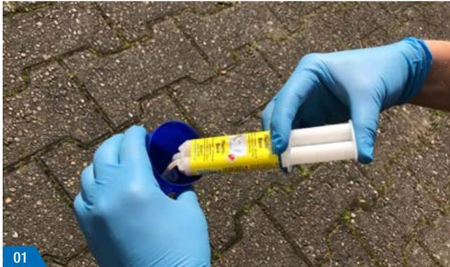
**Step 1:** First, blend the two-component adhesive in a container. Note: Rather blend the mixture a minute too long than too short. Only once you have mixed a homogenous compound, the Plastic-Bond is ready to use.
