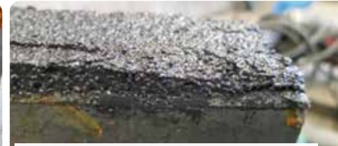
Cross-section of Plastic Metal WP abrasion layer
