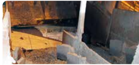
WP - Sag mill chute liner repair & wear protection
