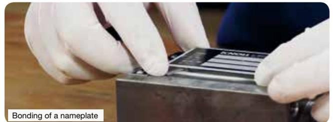
Bonding of a nameplate
