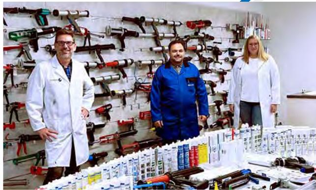
Innotech calls this procedure a portfolio analysis. An adhesive producer provides a large number of products for application tests and the Rettigheim-based company then determines in an extensive test series the best cartridge guns and nozzles for different adhesives.
