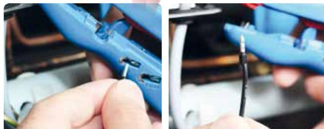
**Pelador de Cable Coaxial No. 1 F Plus**
