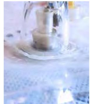
After cleaning, the Easy-Mix RK-7300 was used. First, I put the included mixing nozzle on the cartridge. The RK-7300 is a two-component adhesive, which only turns into a workable compound by means of the helix structure inside of the mixing nozzle. As soon as the adhesive had been applied to the tube material, I fixated the valve by applying gentle pressure. I covered it with a small glass, so it wouldn't accidentally move. Then, Oliver and I allowed the adhesive to cure over night.
