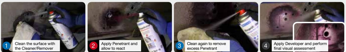
Cleaner, Penetrant and Developer for the non-destructive material testing by way of colour penetration process
